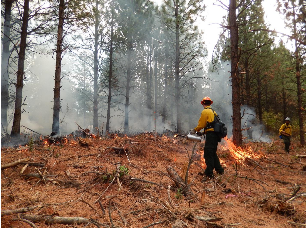
Figure 2. Ignition of instrumented plot in prescribed fire experiments in ponderosa pine stands at the University of Idaho Experimental Forest. Fire intensity was quantified via fire radiative flux density using tower-mounted dual-band infrared radiometers (photo center) and methodology detailed in Kremens et al. (2012).
