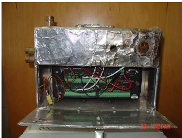
Figure 8—View of Fire Behavior Package datalogger. Logger is accessed through hinged door on package face.
