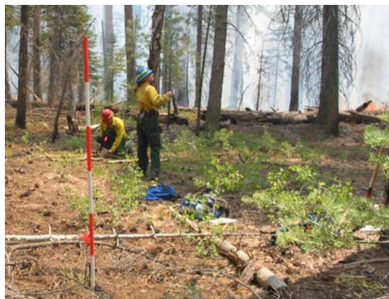
Figure 3. Taking weather observations with sling psychrometer and measuring fuels along a transect.
