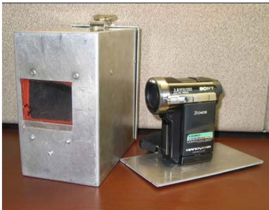
Figure 10—View of digital camera enclosure (10cm X 18cm insulated aluminum) and camera mounting plate.
