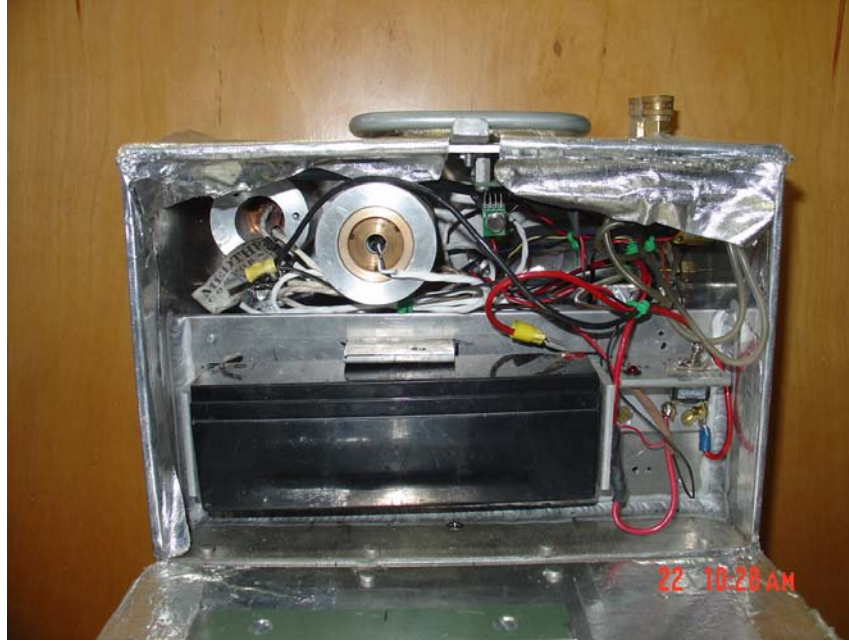
Figure 9—View of Fire Behavior Package battery and electronics, accessed through hinged panel on rear of box. Note aluminum heat sinks for thermal sensors.
