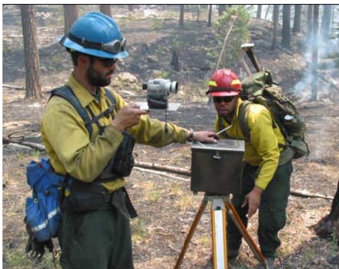
Figure 13—Rapid Response in situ instrumentation team installing the digital camera system on the Dragon WFU Incident.
