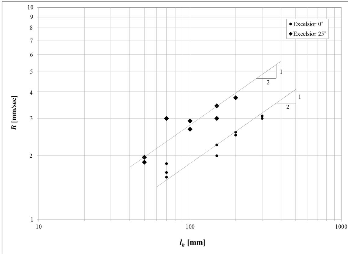
Figure 3. Excelsior trials at two different slopes fit identified convection spread profile.
