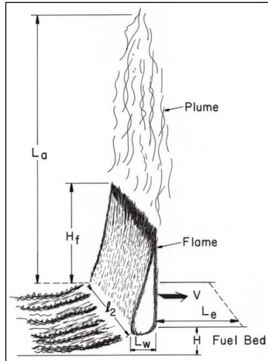
**Figure 1.** Schematic of flame spread over fuel bed and dimensions of flame height, plume height, and fuel bed. [6]
