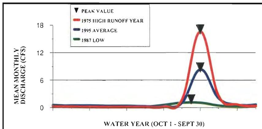
It is important to understand that this chart depicts the runoff characteristics under the current vegetative conditions of a mature forest. Runoff characteristics are expected to be significantly different under different stand conditions resulting from wildfire. The peak discharge values for the above hydrographs are also displayed in Figure III-4 (▼ symbol), Effects by Alternative, to define the lower limit of the range of natural variation for the three levels of runoff.
