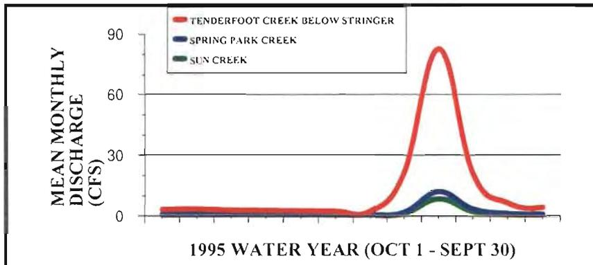
Differences in geology, aspects, and drainage area do create differences in the stream runoff characteristics. The annual and peak discharge of Spring Park Creek is generally higher than Sun Creek because of the slightly larger drainage area and higher elevations that produce slightly higher precipitation levels. The discharge of Tenderfoot Creek, just below Stringer Creek, is higher than the sub-watersheds because of the larger drainage area.
