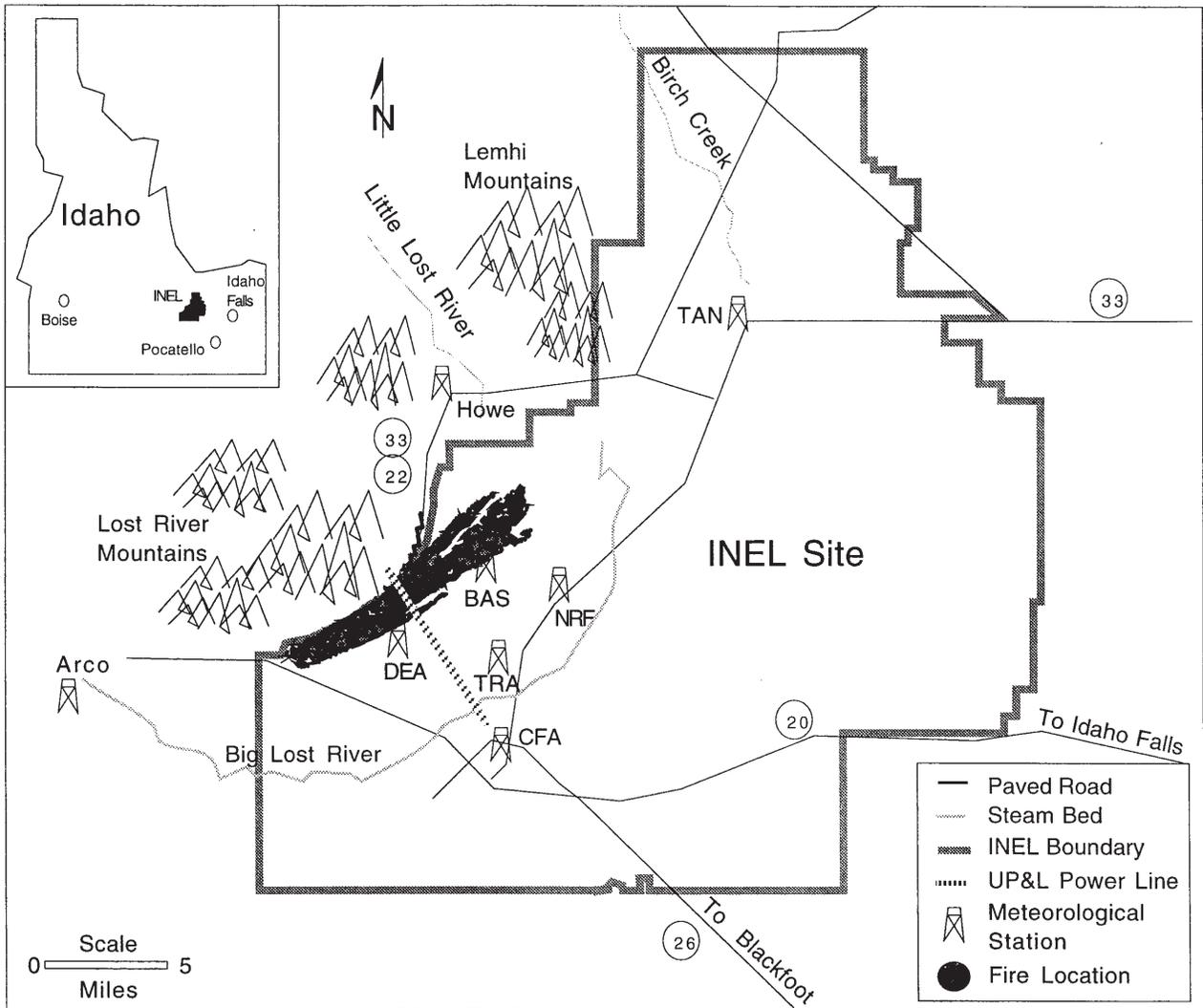
**Figure 1**—Diagram of INEL site and location relative to the State of Idaho. Eight of the meteorological stations are shown (scale is approximate). Arco and Howe stations' names come from the towns where they are located. Six acronyms stand for: DEA-Dead Man Canyon; BAS-Base of Howe Peak; TAN-Test Area North; CFA-Central Facilities Area; NRF-Naval Reactor Facility; TRA-Test Reactor Area.
